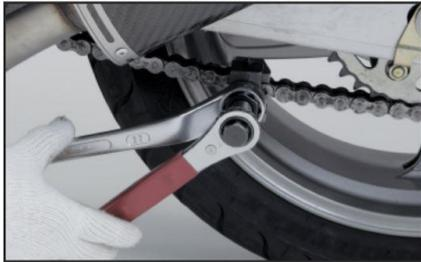
4. Using a spanner and ratchet, slowly tighten the splitting pin whilst holding the tool in place to keep the splitting pin aligned.
