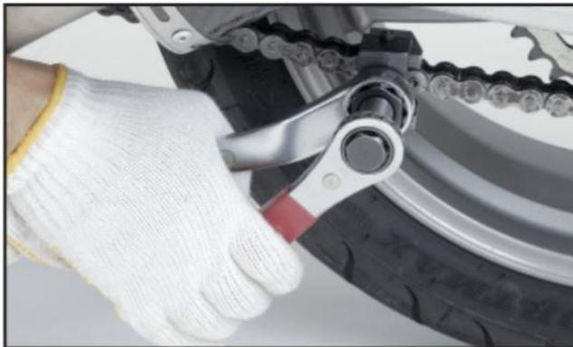
3. Using the same method as previous, hold the tool in place with a spanner and tighten the tool with a wrench until the sides of the rivet pin makes contact with the link plate.
