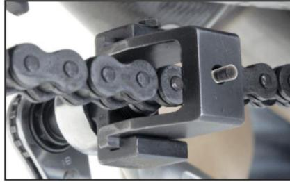
5. Keep winding in the tool until the chain pin is completely removed from the links. The chain is now split.
