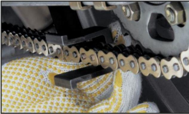
1. Place the U-Shaped part of the tool over the link making sure the pins on the back part of the link are sat in the groove of the tool.
