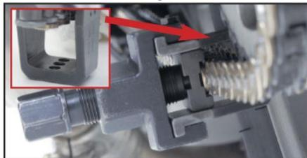
3. Place the U-Shaped part of the tool over the new link and line up the dimples with the chain pins. Put the plate holder in position and flip the pin over to the rivet side.
