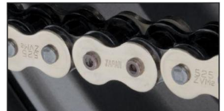
5. Once the plate is in place, you can now fit the split link (with the closed end face direction of travel) or in case of rivet links, the next step is to flare out the rivet pin.
