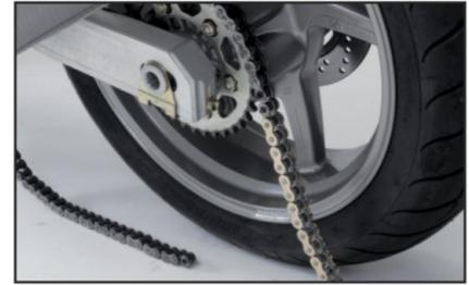
6. Remove the chain from the bike or any of the excess links when cutting down a chain.
