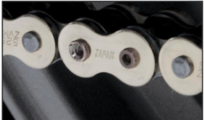
4. Above is an image of a properly flared chain pin. If the link isn't flared as much as the pin on the left, then realign the tool and repeat the process. Any cracks or splits in the pin will mean a new link is needed.
