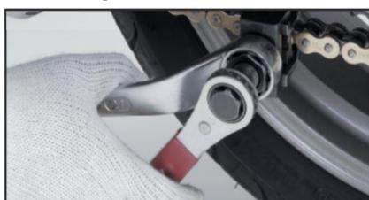
4. Using the same method as splitting the chain, hold the tool in place with a spanner and use a ratchet to tighten the tool up and press the new plate onto the link.
