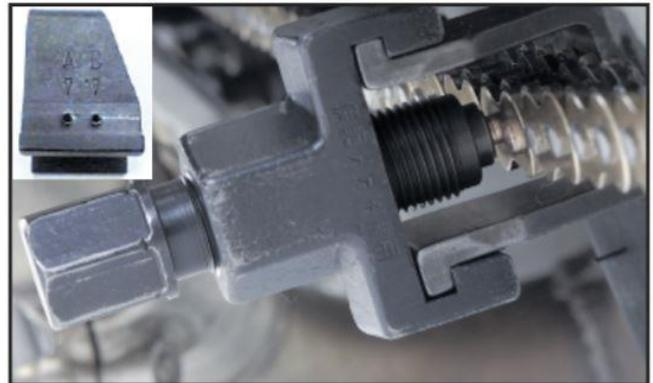
2. Put the rest of the chain tool in position using the rivet end of the splitting tool. Make sure that the rivet side of the tool is sat flush on the pin that need to be flared.
